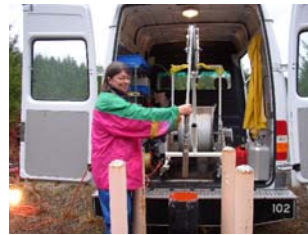
Pam Bennett-Cumming testing a monitoring well.
